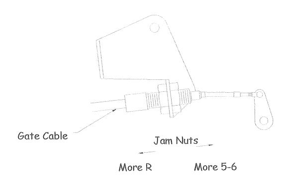
Small adjustments (1/6 of a turn) made with both jam nuts makes a noticeable difference. A smooth shift sequence is therefore attainable first through fourth gears and reverse.
